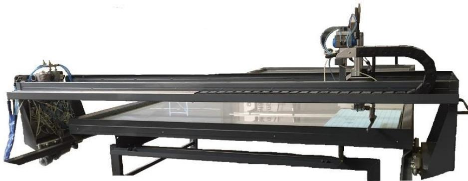
The application width (Y-axis) can be adjusted step less from 1000mm to 2900mm, by adjusting simple on/off lever switches. The traverse speed can be adjusted. The maximum traverse speed is 26m/min with a 500mm single row spreader. The bonding speed is adjusted in accordance with the Y-axis speed in order to obtain exact coverage of the adhesive layer. The bonding speed is depending on the actual oscillating time for the individual panel width.
